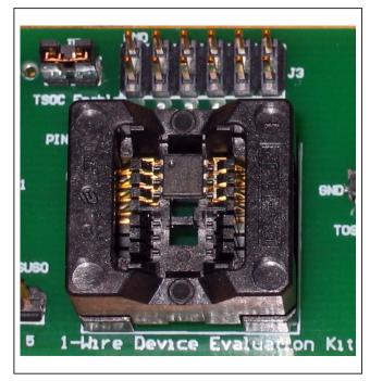
Figure 4. TSOC Package Insertion
