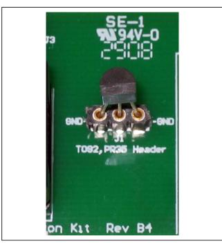
Figure 3. TO92/PR35 Package Insertion
